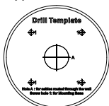
Figure 2-15 Drill Template of the Junction Box
