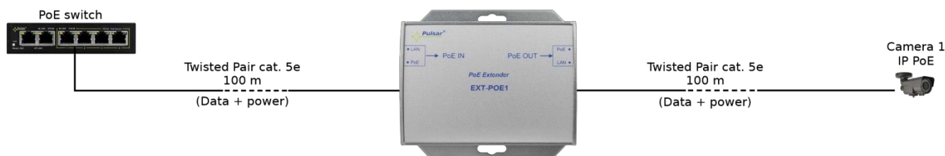
Extension of the IP PoE camera range by 100 m
